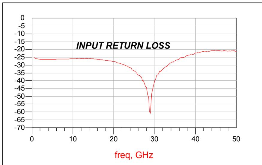
Typical Performance ( On Wafer Measurements )
