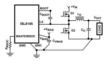
FIGURE 8. PRINTED CIRCUIT BOARD SMALL SIGNAL LAYOUT GUIDELINES
