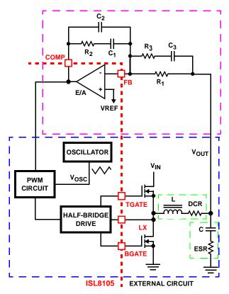
FIGURE 9. VOLTAGE-MODE BUCK CONVERTER COMPENSATION DESIGN
