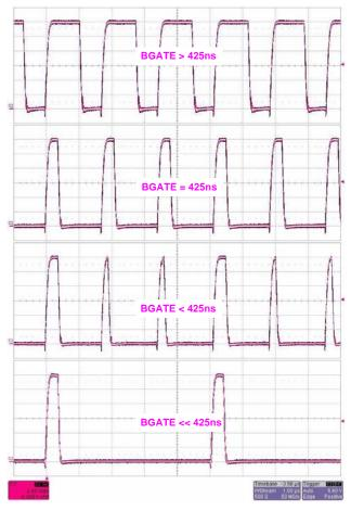
FIGURE 4. BGATE PULSE STRETCHING
