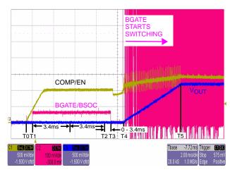
FIGURE 2. BGATE/BSOC AND SOFT-START OPERATION
