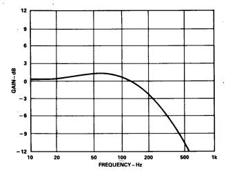
ever, an increasing bandwidth also leads to an increase in the susceptibility to noise, as the higher frequency noise signals come into the range of frequencies "seen" by the converter (remember that the converter is effectively a low pass filter). One of the major detrimental effects of this increase in the susceptibility to noise, is the appearance of the noise on the analog velocity output signal.
