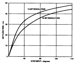
It can be seen that for step inputs within approximately 5-10 degrees, the response is linear, and can be derived from the small signal response of the converter (i.e., see bandwidth). Beyond this region, the internal error voltage will exceed the linear range of the converter.
