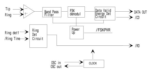
Fig.13 FSK Block Diagram
