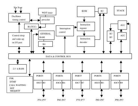
Fig.3 Block diagram2
