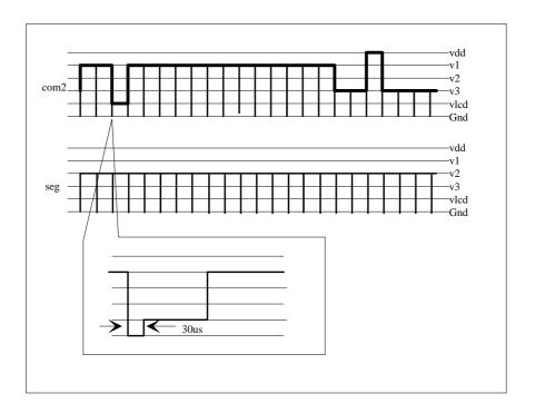
Fig.11 key scan signal
