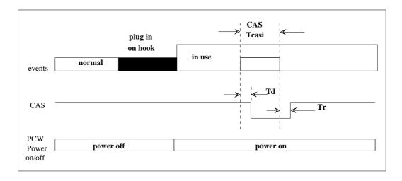
Fig.20 Call Waiting Timing Diagram
