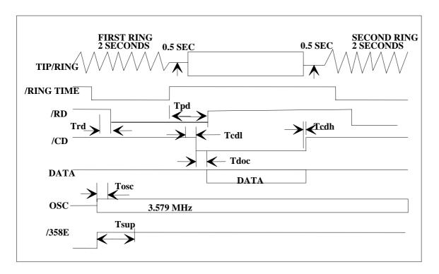
Fig.19 FSK Timing Diagram
