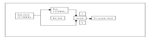
Fig.8 The relation between 32.768kHz and 3.579MHz.
