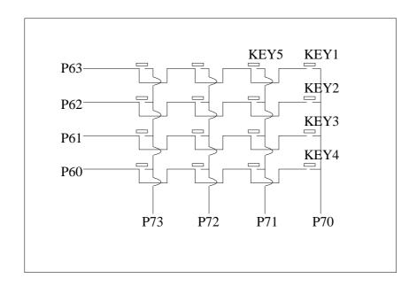
Fig.10 Key scan circuit
