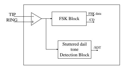
Fig.17 Stuttered dial tone block diagram
