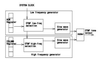
Fig.15 DTMF Block Diagram
