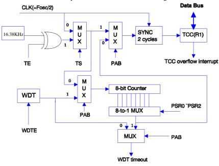
Fig. 10 Block diagram of TCC WDT
