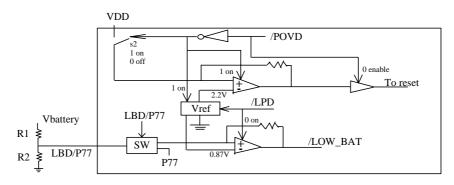
Fig.7 Universal low battery detect with /LPD,/POVD and /LOW\_BAT
