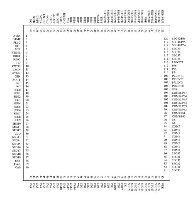
Fig1. Pin Assignment
