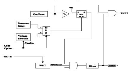
Fig.12 Block diagram of Reset of controller
