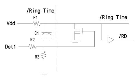
Fig.14 ring detect circuit
