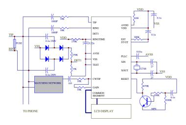
Note: If FSK sensitivity is poor, user can connect 1M ohms resistor between TIP pin and RING pin.
