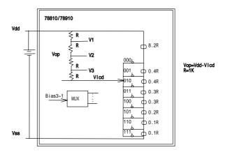
Fig.18 LCD bias circuit
