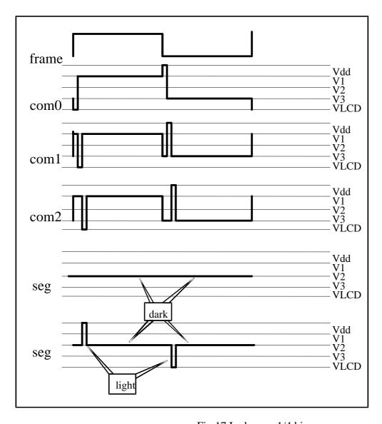
Fig.17 Lcd wave 1/4 bias
