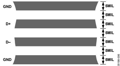
Figure 18. Arrangements of Signal Tracks
