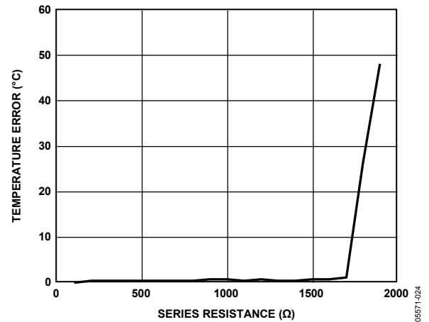
Figure 14. Temperature Error vs. Series Resistance
