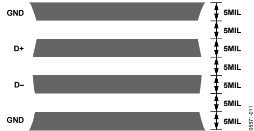
Figure 23. Typical Arrangement of Signal Tracks
