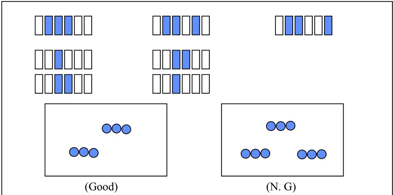
Fig. 3. Minimum distance between dot defects
