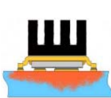
⑨ Mounted on minimum footprint full size board with metalized back and with small clip heatsink. (still air)
