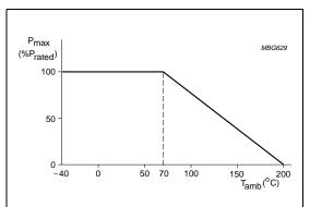
Fig.1 Maximum dissipation ( $P_{max}$ ) as a function of the ambient temperature ( $T_{amb}$ ).
