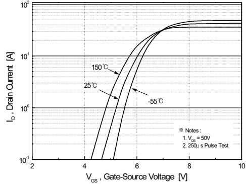
Figure 2. Transfer Characteristics
