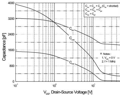
Figure 5. Capacitance Characteristics
