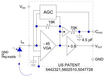
Photodector cathode must be connected to  $I_{\text{IN}}$  for proper AGC operation
