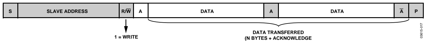
Figure 17. I 2 C—Master Reading Data from Slave
