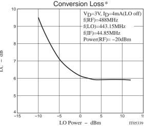
\* This Conversion Loss characteristic includes the loss of the test board and the Balun Transformer.
