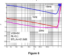
Total Harmonic Distortion Plus Noise vs Frequency
