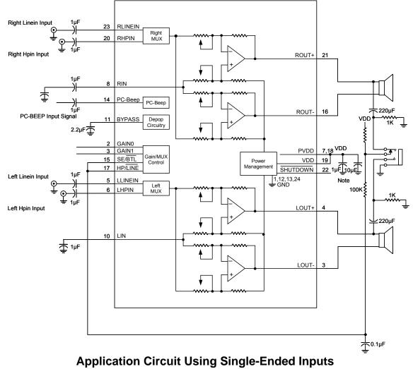
Note: 1µF ceramic capacitor should be placed as close as possible to the IC to filter the higher-frequency noise.
