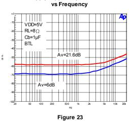
**Supply Ripple Rejection Ratio**
