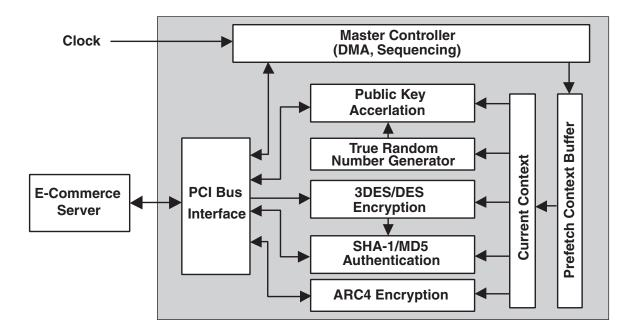
The BCM5820 integrates into a single 256-BGA package 4x–5x the public-key performance of competing board level products at a fraction of the cost. The BCM5820 device's 32/64 33- to 66-MHz PCI interface makes it a perfect solution for add-in card applications for high performance E-commerce servers, load balancing, and web switching equipment.
