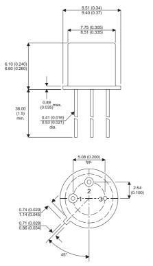
Bipolar NPN Device in a Hermetically sealed TO5 Metal Package.
