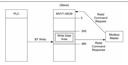
**Ex. 2** -- The next figure shows another example of how to use the Write Data Area; an MVI71-MCM port configured as a Master sends a Modbus Write Command to a slave device. The Modbus Write Command source address in the MVI71-MCM database must be located inside the Write Data Area (between addresses 240 and 479).
