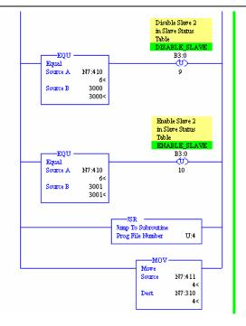
This rung will only execute when a BTR or BTW message is not enabled. This logic is required to alternate between the BTR and BTW messages. When it is time to perform a BTR operation, the 64-word data block will be transferred to N7:410. The remaining branches of the rung then process this data.
