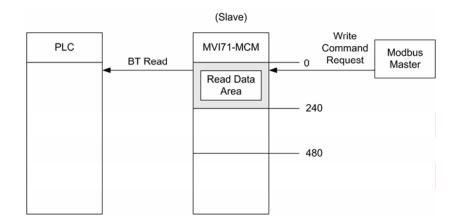
**Ex. 2** -- The next figure shows another example of how to use the Read Data Area; an MVI71-MCM port configured as a Master sends a Modbus Read Command to a Slave device. The Modbus Read Command destination address must be located inside the Read Data Area (between addresses 0 and 239).
