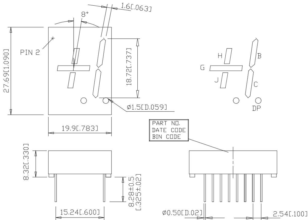
NOTES: All dimensions are in millimeters. Tolerances are ± 0.25 mm (0.01") unless otherwise noted.
