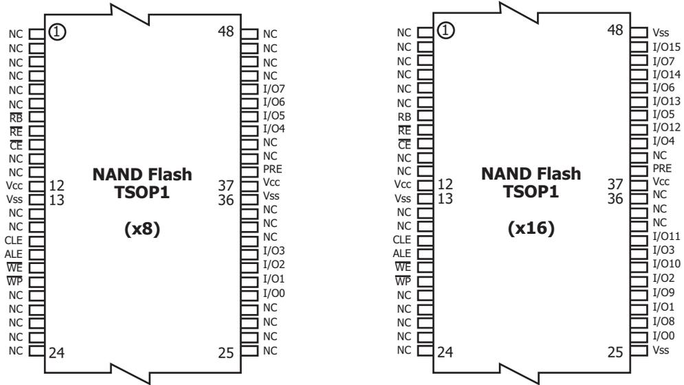
Figure 2. 48TSOP1 Contactions, x8 and x16 Device
