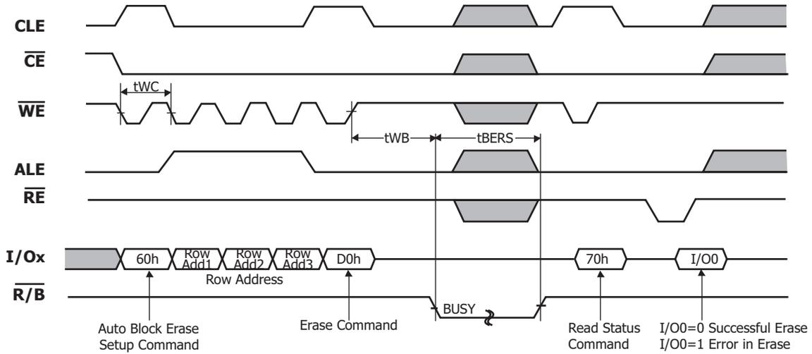
**Figure 16: Block Erase Operation (Erase One Block)**
