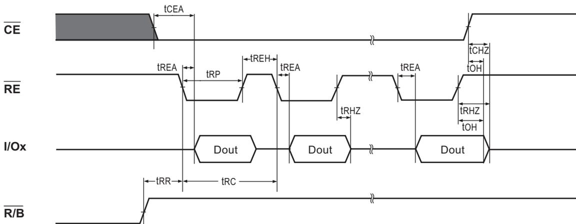
**Figure 7: Sequential Out Cycle after Read (CLE=L, WE#=H, ALE=L)**
