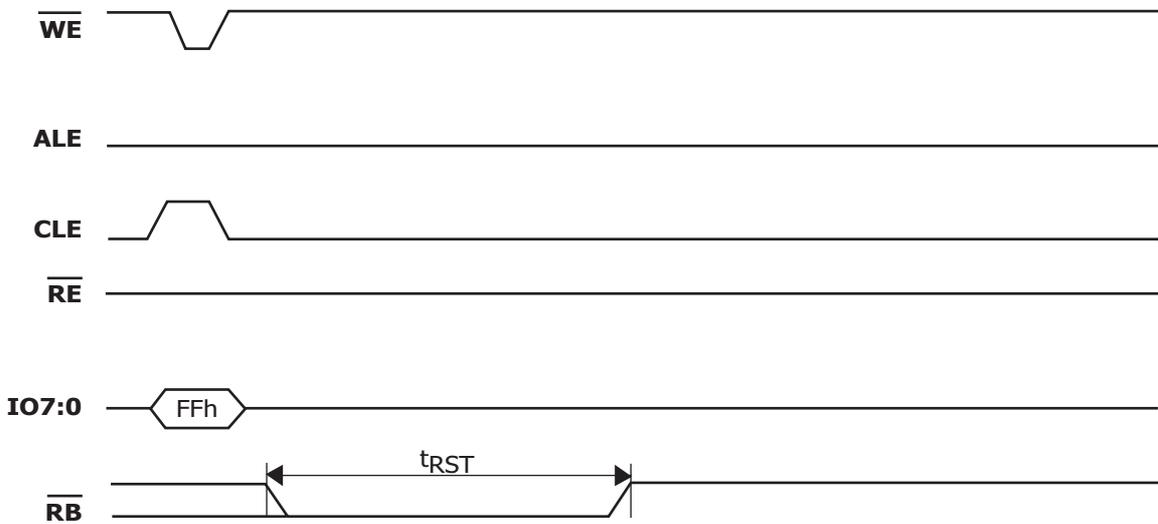
Figure 22: Reset Operation
