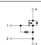
Please use the S1 pin for gate input signal return. Make sure that the main current
