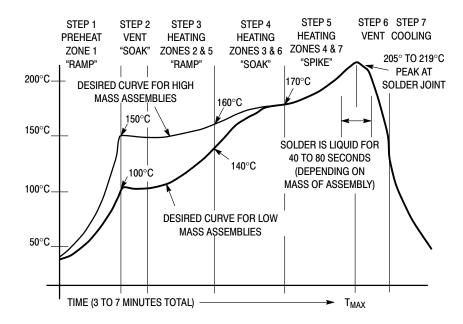
Figure 1. Typical Solder Heating Profile
