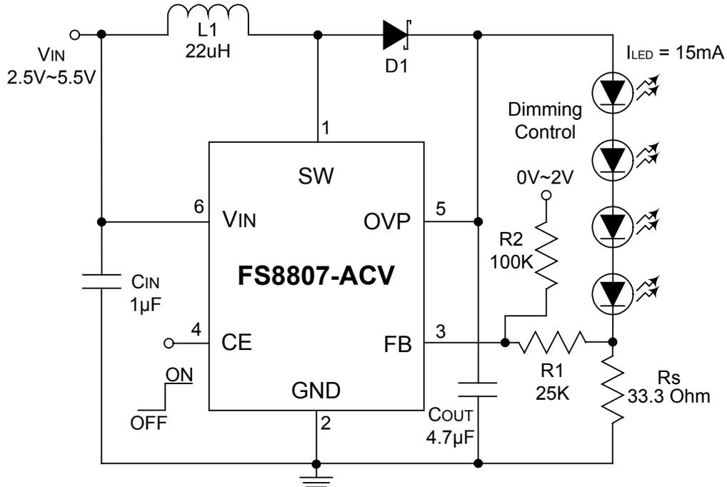
Fig 3. White LED application with DC voltage dimming control
