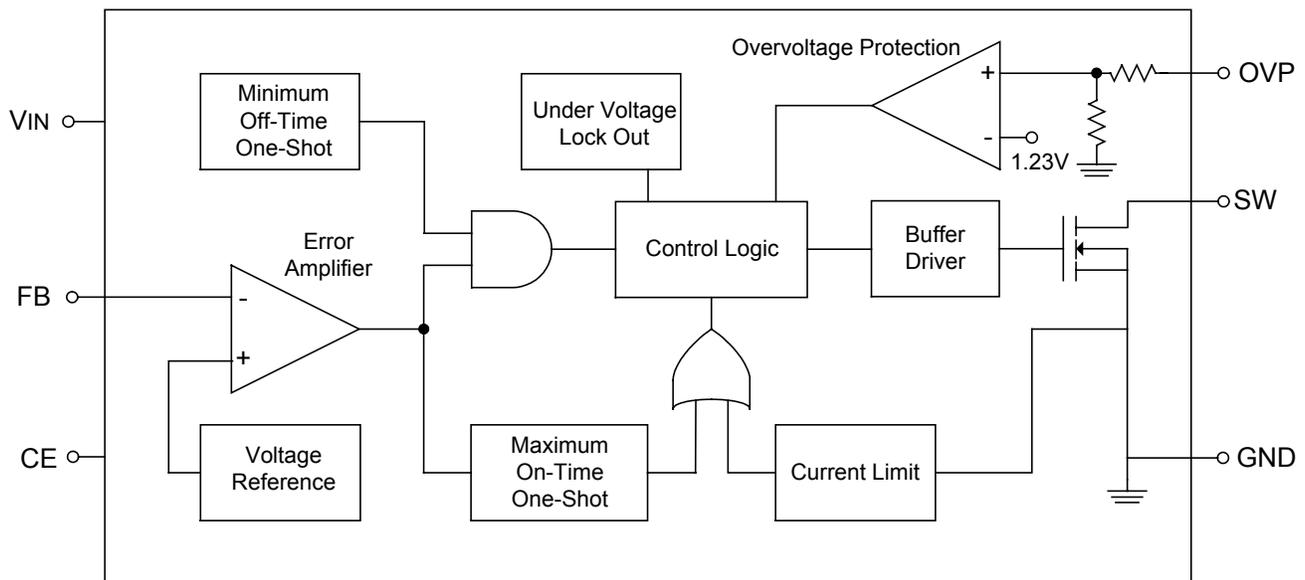
Fig 2. FS8807 Simplified Functional Block Diagram
