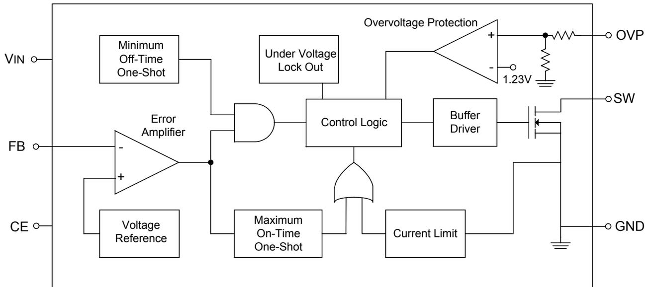
Fig 2. FS8807 Simplified Functional Block Diagram
