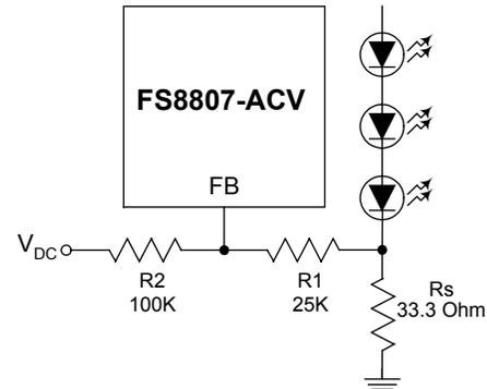
For  $V_{DC}$  range from 0V to 2V, the selection of resistors in this figure gives dimming control of LED current from 0mA to 15mA. Following steps are used to select the resistor values:
