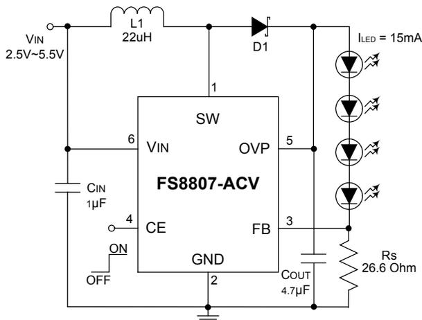
Fig 1. FS8807 Typical Application for driving 4 White LEDs
