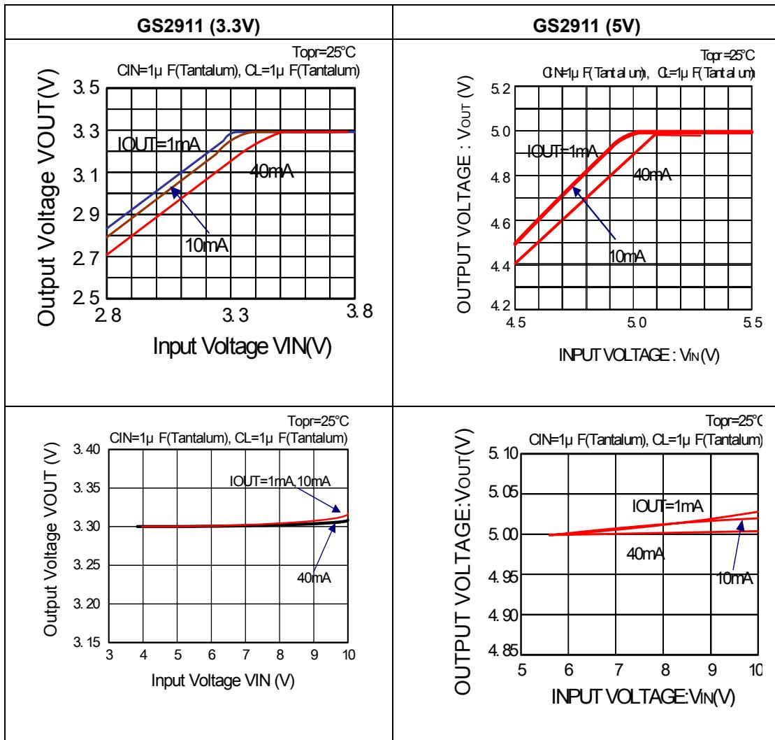
**Input/Output Voltage Differential vs. Output Current**
