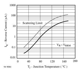
Figure 1. Reverse Current vs. Junction Temperature
