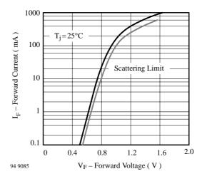
Figure 2. Forward Current vs. Forward Voltage
