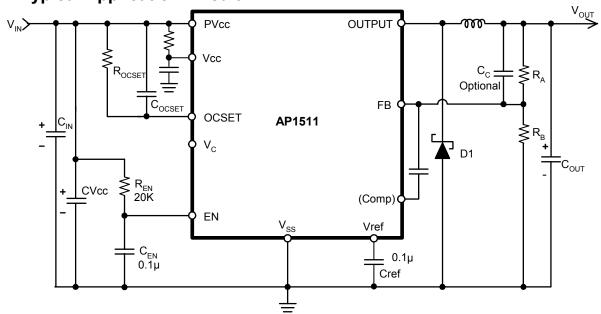
Note:  $V_{OUT} = V_{REF} \times (1+R_A/R_B)$ R<sub>B</sub>=1K~10K ohm
