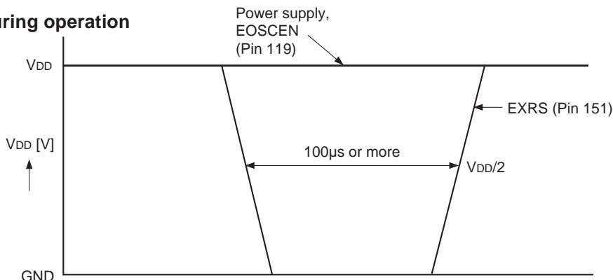
For initialization during operation, the interior circuit except internal RAM is initialized by setting the EXRS (Pin 151) signal to the low level for 100 $\mu$ s or more. Note that internal RAM is not also initialized by the operation. At this time, the EOSCEN (Pin 119) signal should keep the high level.
