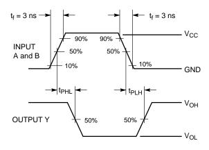
Figure 3. Switching Waveform
