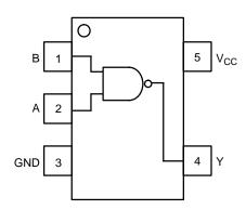
Figure 1. Pinout (Top View)
