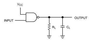
A 1–MHz square input wave is recommended for propagation delay tests.
