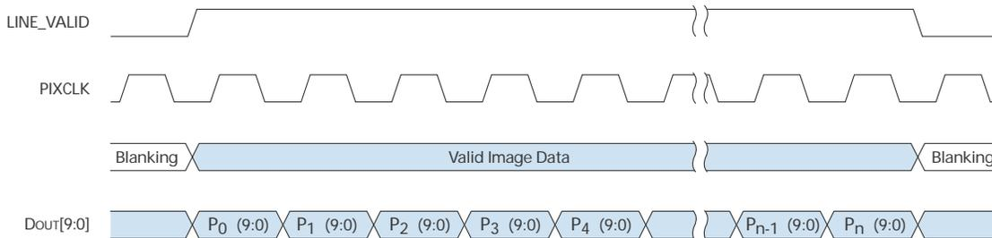
**Figure 8: Row Timing and FRAME\_VALID/LINE\_VALID Signals**
