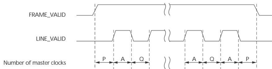
The sensor timing (Table 3) is shown in terms of pixel-clock and master-clock cycles (see Figure 7 on page 10). The recommended master clock frequency is 36 MHz. Increasing the integration time to more than one frame will cause the frame time to be extended. The equations in Table 3 assume integration time is less than the number of rows in a frame ( $\text{Reg0x09} <$
