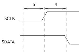
**Figure 36: Serial Host Interface Stop Condition Timing**
