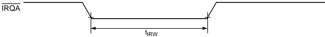
Figure 10-6 External Interrupt Timing (Negative-Edge-Sensitive)
