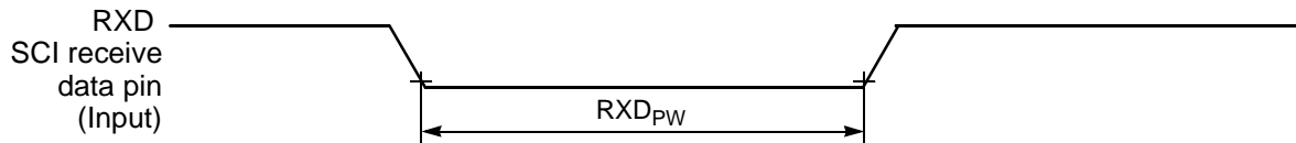
Figure 10-15 RXD Pulse Width
