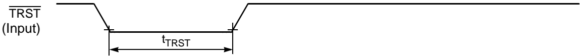
Figure 10-20 \overline{TRST} Timing Diagram (This pin is always tied inactive on the 56F8322)
