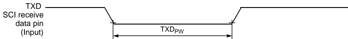
Figure 10-16 TXD Pulse Width
