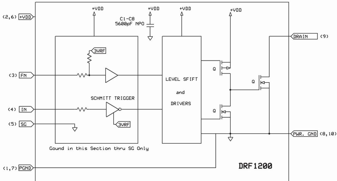
Figure 1, DRF1200 Simplified Circuit Diagram
