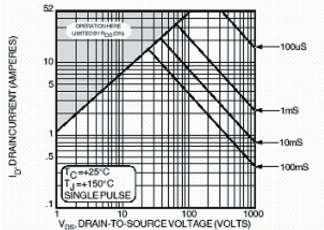
Figure 6, Typical Maximum Safe Operating Area
