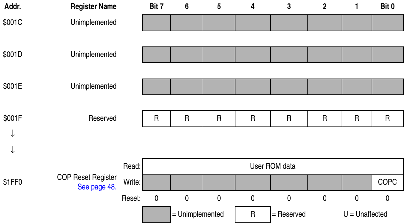
Figure 2-2. Input/Output Registers (Sheet 4 of 4)
