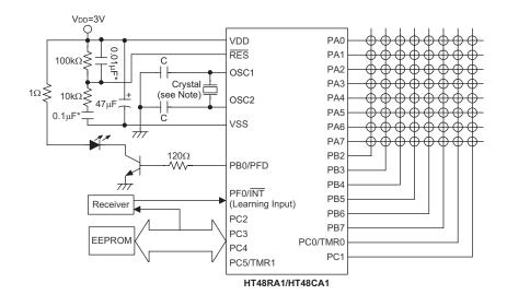
Note: The resistance and capacitance for reset circuit should be designed to ensure that the VDD is stable and remains in a valid range of the operating voltage before bringing RES to high.
