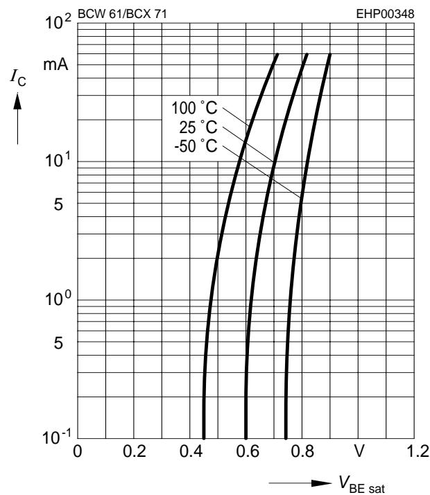
**Collector current**  $I_C = f(V_{BE})$
