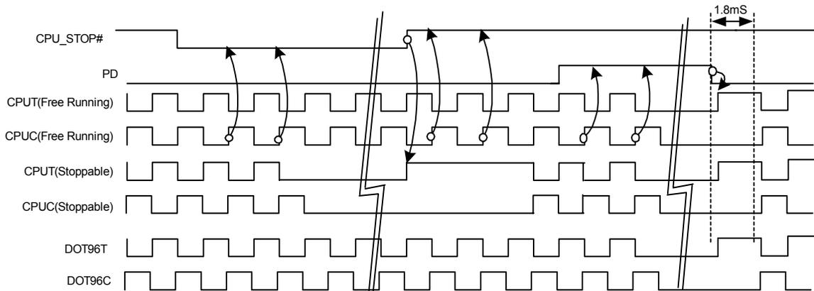
**Figure 9. CPU\_STOP# = Tri-state, CPU\_PD = Tri-state, DOT\_PD = Tri-state**
