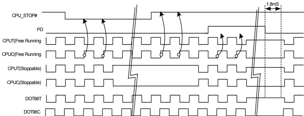
**Figure 8. CPU\_STOP# = Driven, CPU\_PD = Driven, DOT\_PD = Driven**
