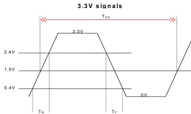
**Figure 16. Single-ended Output Signals (for AC Parameters Measurement)**
