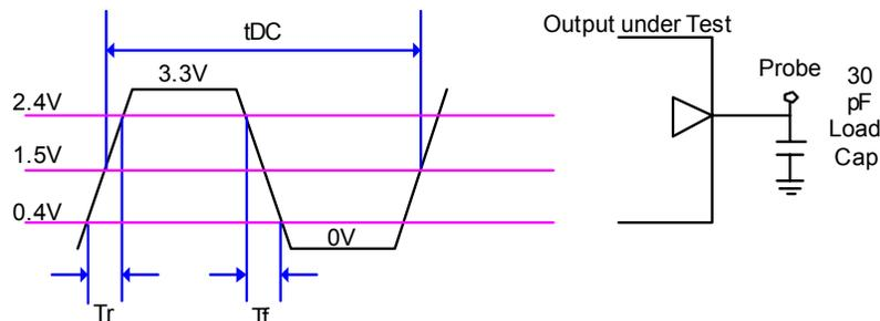
**Figure 14. Single ended PCI lumped load configuration**
