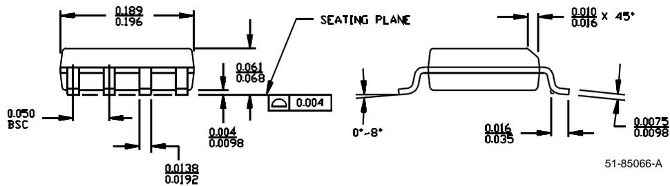
16-lead (150-Mil) Molded SOIC S16
