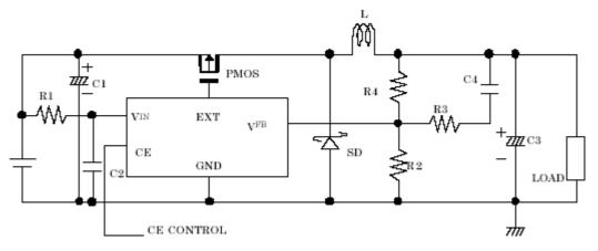
PMOS: SI9435 L: 27  $\mu$  H SD1: 1N5817 C1: 10  $\mu$  F (Ceramic Type or Electrolytic Type) C2: 0.1  $\mu$  F (Ceramic Type or Electrolytic Type) C3: 47  $\mu$  F (Tantalum Type) C4: 1000pF (Ceramic Type) R1=10  $\Omega$ , R2=14.3k  $\Omega$ , R3=2.7k  $\Omega$ , R4=33k  $\Omega$
