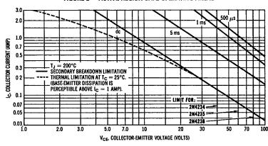
The Safe Operating Area Curves indicate Ic — Vce limits below which the device will not enter secondary breakdown. Collector load lines for specific circuits must fall within the applicable Safe Area to avoid causing a catastrophic failure. To insure operation below the maximum T<sub>1</sub>, power-temperature derating must be observed for both steady state and pulse power conditions.
