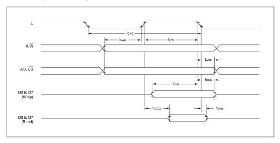
Note: tcyc6 indicates the interval during which  $\overline{\text{CS}}$  is LOW and E is HIGH.
