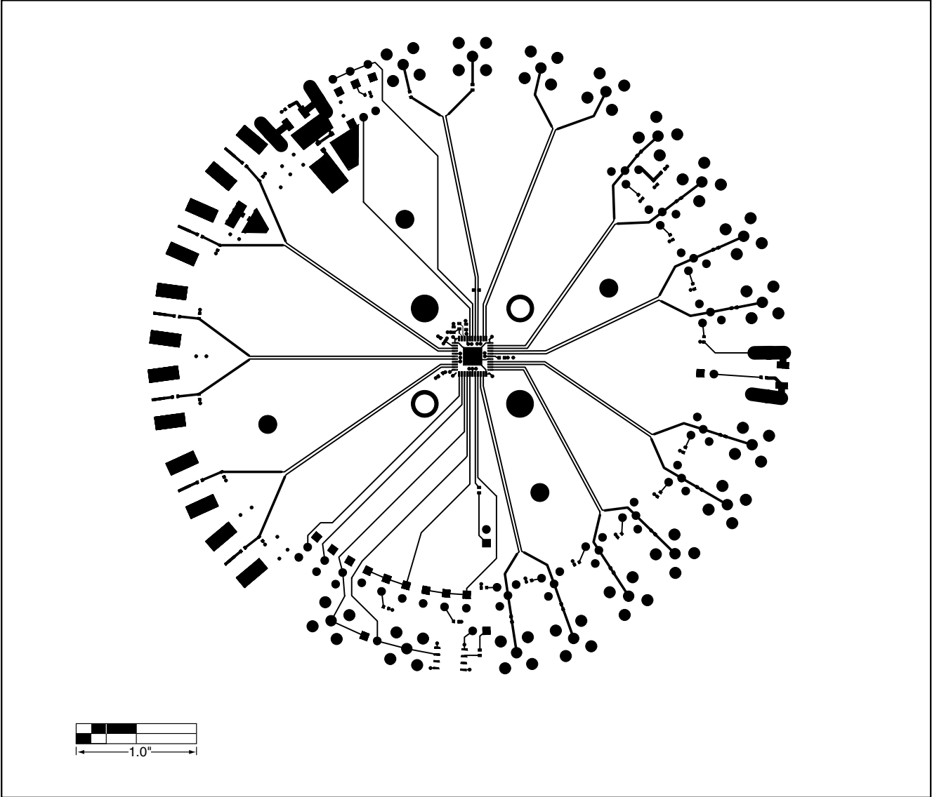
Figure 4. MAX3892 EV Kit PC Board Layout—Component Side
