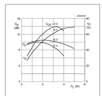
Pulsed, class-AB; f = 900 MHz;  $I_{CQ}$  = 2 mA; tuned at  $P_L$  = 3.5 W;  $T_{s} \leq 60~^{\circ}\text{C}.$
