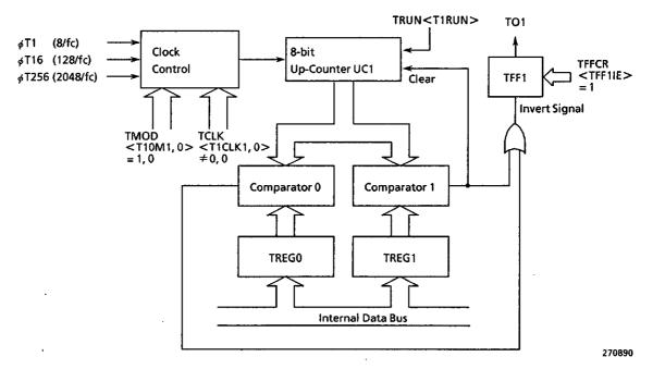
Figure 3.6 (10) Block Diagram of 8-bit PPG Mode
