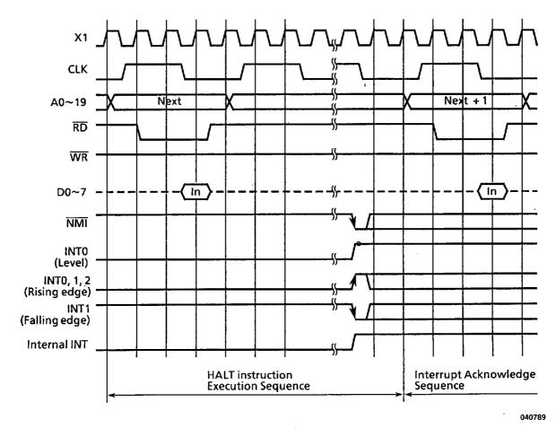
Figure 3.4 (2) Timing Chart for Releasing the HALT State by Interrupts in RUN/IDLE 2 Modes
