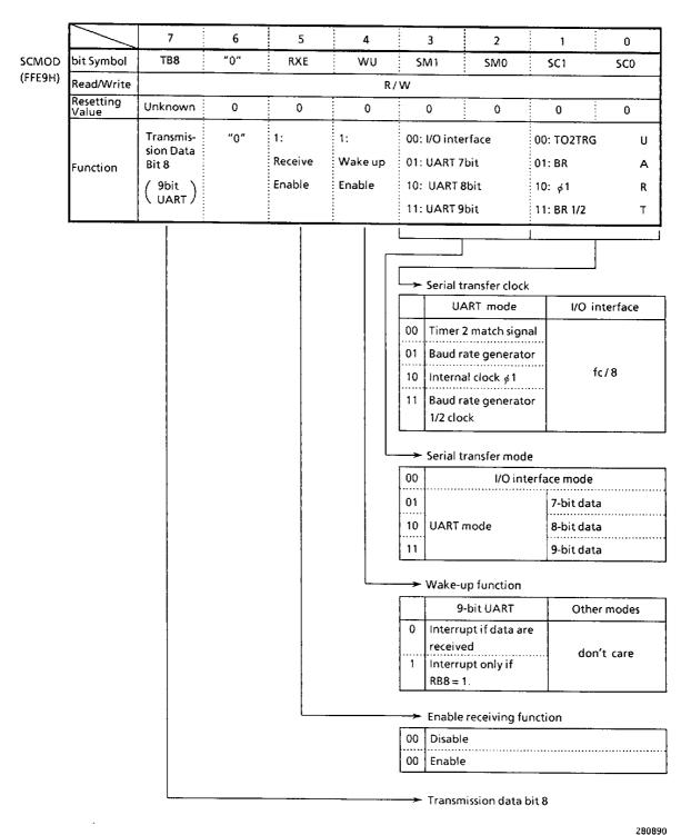
Figure 3.8 (2) Serial Channel Mode Register
