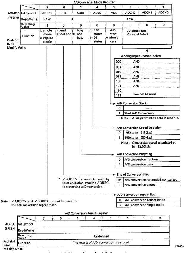
Figure 3.9 (2) Registers for A/D Conversion
