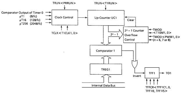
Figure 3.6 (11) Block Diagram of 8-bit PWM Mode
