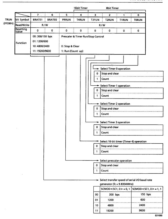
Figure 3.6 (5) Timer/Serial Channel Control Registers TRUN
