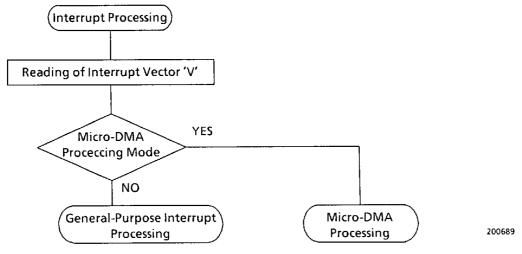
Figure 3.3 (1) Interrupt Response Flowchart
