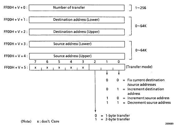
Figure 3.3 (4) Parameters for Micro DMA Processing
