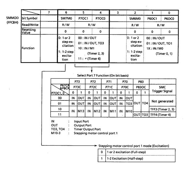
Figure 3.7 (26) Stepping Motor Control Port Mode Registers
