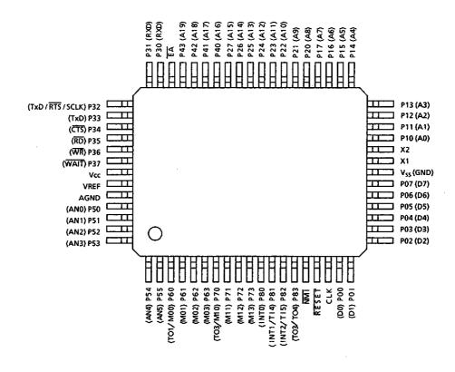
Figure 2.1-(2) Pin Assignment (Flat Package)
