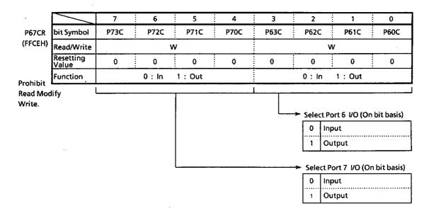
Figure 3.7 (1) Ports 6 and 7 I/O Selection Registers
