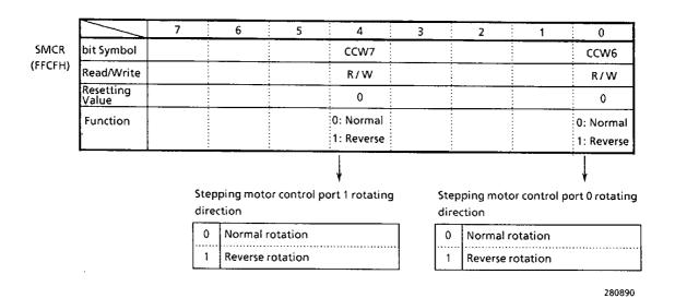
Figure 3.7 (3) Stepping Motor Control Port Rotating Direction Control Registers
