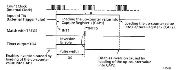
Figure 3.6 (19) One-Shot Pulse Output (with no delay)
