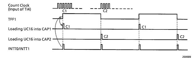
Figure 3.6 (20) Frequency Measurement
