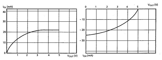
Figure 4.11 (4) VOUT - IOL TYPICAL CURVE
