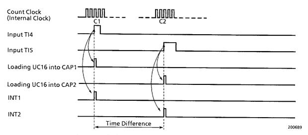
Figure 3.6 (22) Time Difference measurement
