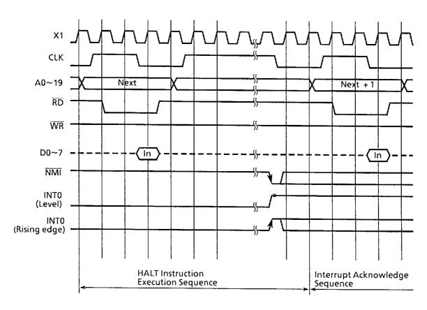
Figure 3.4 (3) Timing Chart of HALT Released by Interrupts in IDLE1 Mode
