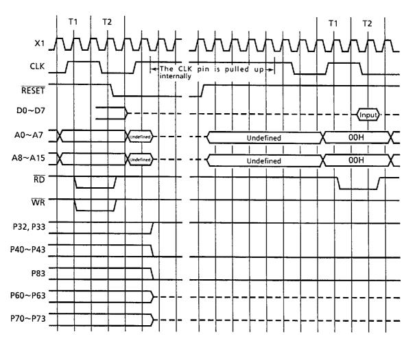
Figure 3.1 (1b) TMP90C841A Reset Timing
