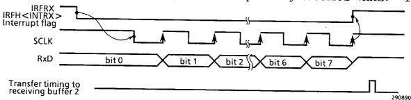
Figure 3.8 (13) Receiving Operation (I/O Interface Mode)
