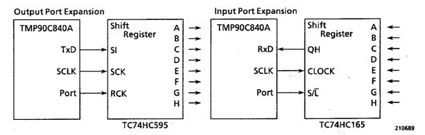
Figure 3.8 (11) I/O Interface Mode
