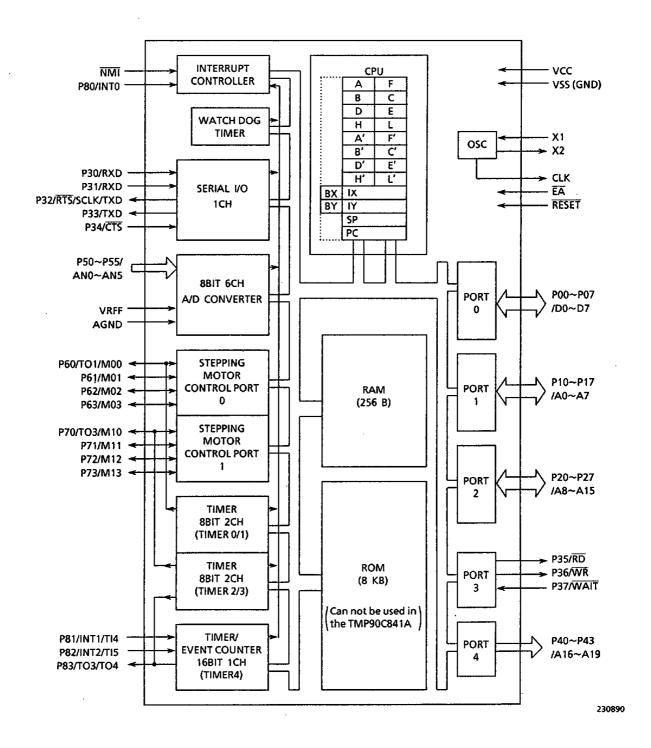
Figure 1 TMP90C840A Block Diagram
