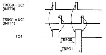
In the 8-bit PPG mode, programmable pulse is generated by the inversion of the timer output each time the 8-bit up-counter 1 (UC1) matches the timer register TREGO or TREG1.
