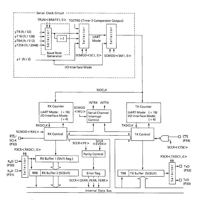
Fifure 3.8 (7) Block Diagram of Serial Channel
