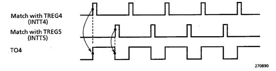
Figure 3.6 (17) Programmable Pulse Output
