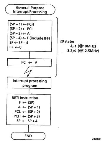
Figure 3.3 (2) General Purpose Interrupt Processing Flowchart
