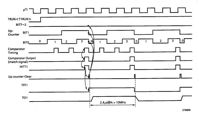
Figure 3.6 (7) Pulse Output (50% duty) Timing Chart
