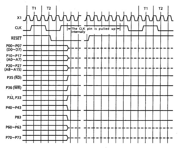
Figure 3.1 (1a) TMP90C840A Reset Timing
