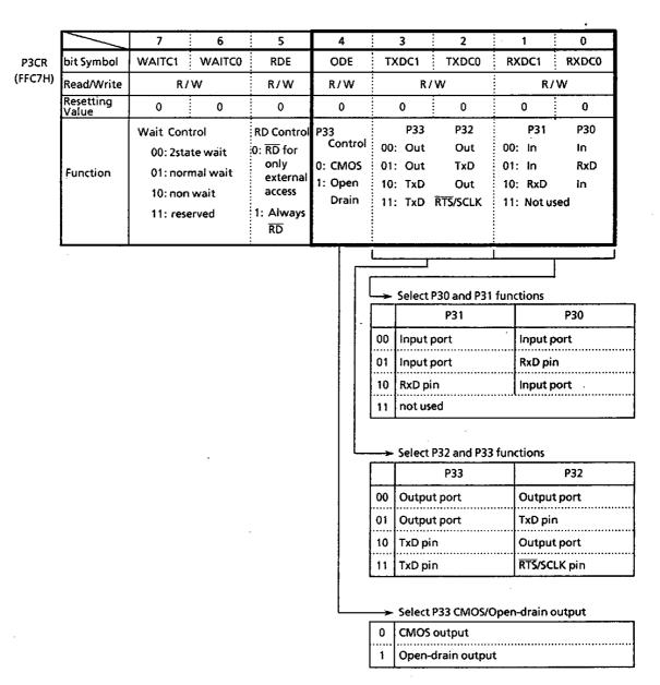
Figure 3.8 (6) Port 3 Control Register
