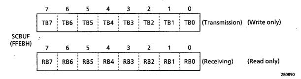
Figure 3.8 (4) Serial Transmission/Receiving Buffer Registers
