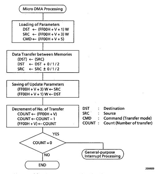
Figure 3.3 (3) Micro DMA Processing Flowchart
