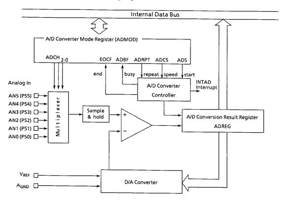
Figure 3.9 (1) Block Diagram of A/D Converter
