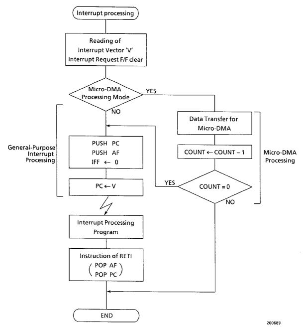
Figure 3.3 (6) Interrupt Processing Flowchart
