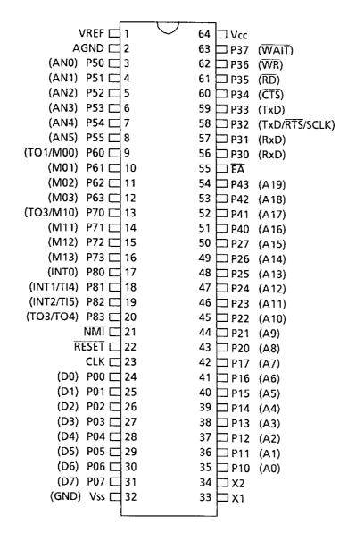
Figure 2.1- (1) Pin Assignment (Shrink Dual Inline Package)
