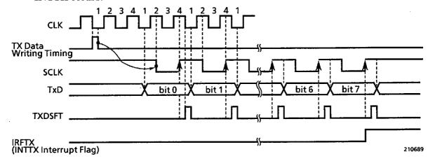
Figure 3.8 (12) Transmitting Operation (I/O Interface Mode)
