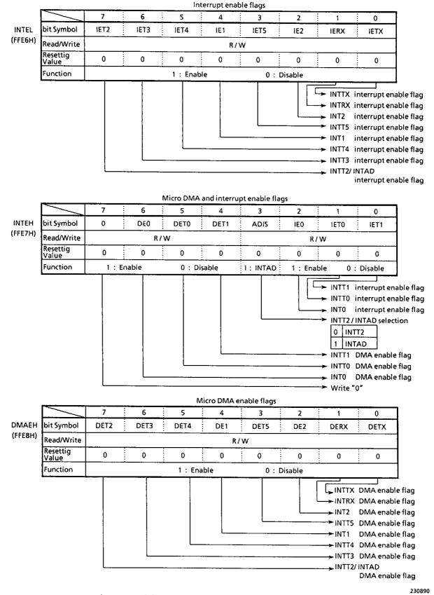
Figure 3.3 (9) Interrupt/Micro DMA Enable Flags
