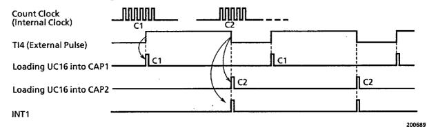
Figure 3.6 (21) Pulse Width Measurement
