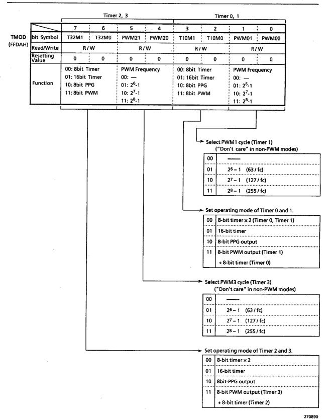
Figure 3.5 (3) 8-bit Timer Mode Register TMOD
