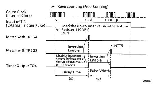
Figure 3.6 (18) One-Shot Pulse Output (with delay)
