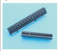
The card-edge connectors utilize an "eye-of-needle"-compliant section for termination to a backplane. The press-fit connectors are targeted for use on 2.36mm (0.093") to 4.19mm (0.165") thick PCBs. By using press-fit connectors, manufacturers can avoid soldering problems and improve manufacturing yields when implementing I/O slots on thick backplanes. RoHS-compliant connector versions are available.
