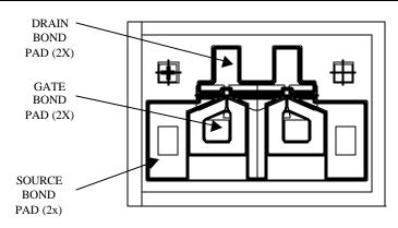
DIE SIZE: 18.0X13.0 mils (460x330  $\mu m)$  DIE THICKNESS: 3.9 mils (100  $\mu m)$  BONDING PADS: 1.9X1.9 mils (50x50  $\mu m)$
