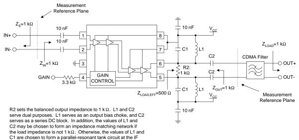
when the IF filter's input impedance is 1 k  $\Omega$ .
