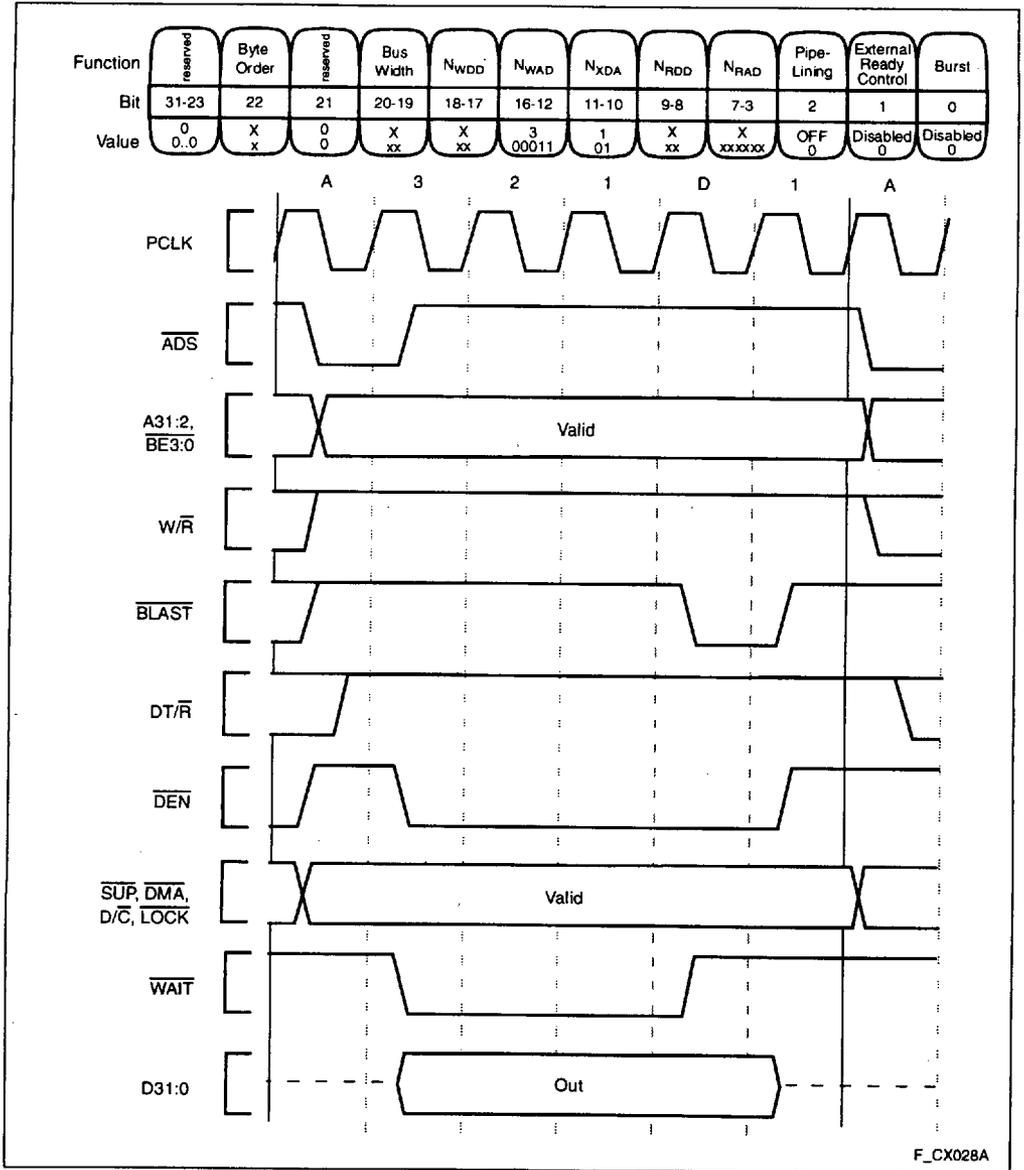
Figure 26. Non-Burst, Non-Pipelined Write Request With Wait States
