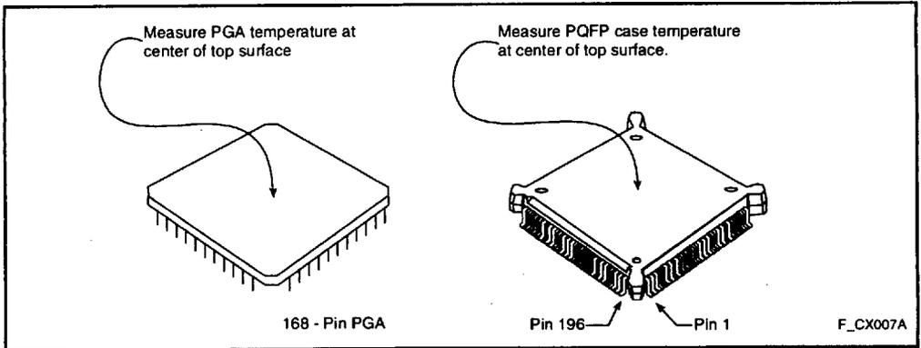
Figure 5. Measuring 80960CA PGA and PQFP Case Temperature
