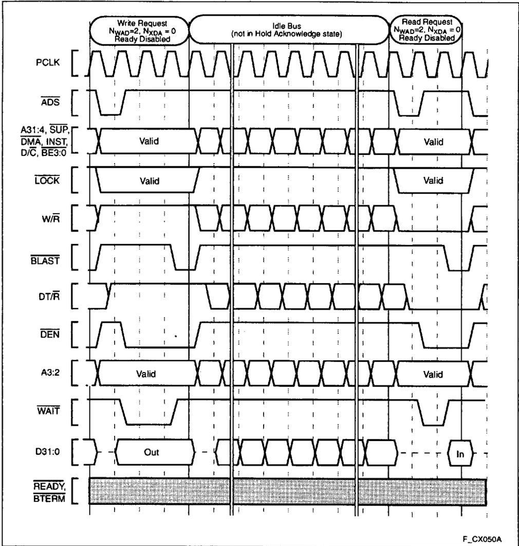
Figure 49. Idle Bus Operation
