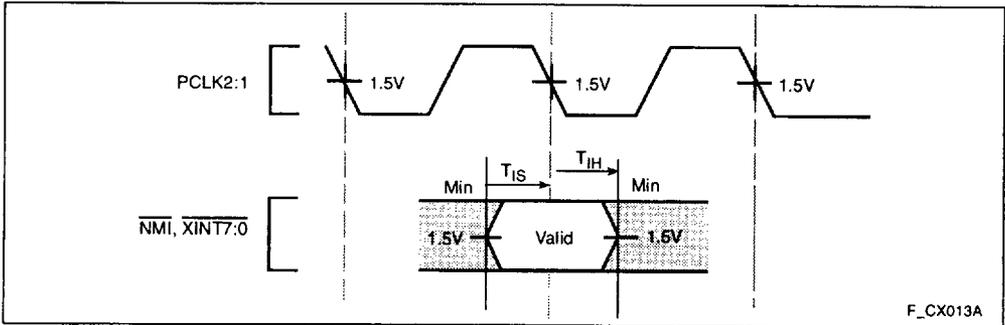
Figure 12. NMI, XINT7:0 Input Setup and Hold Waveform
