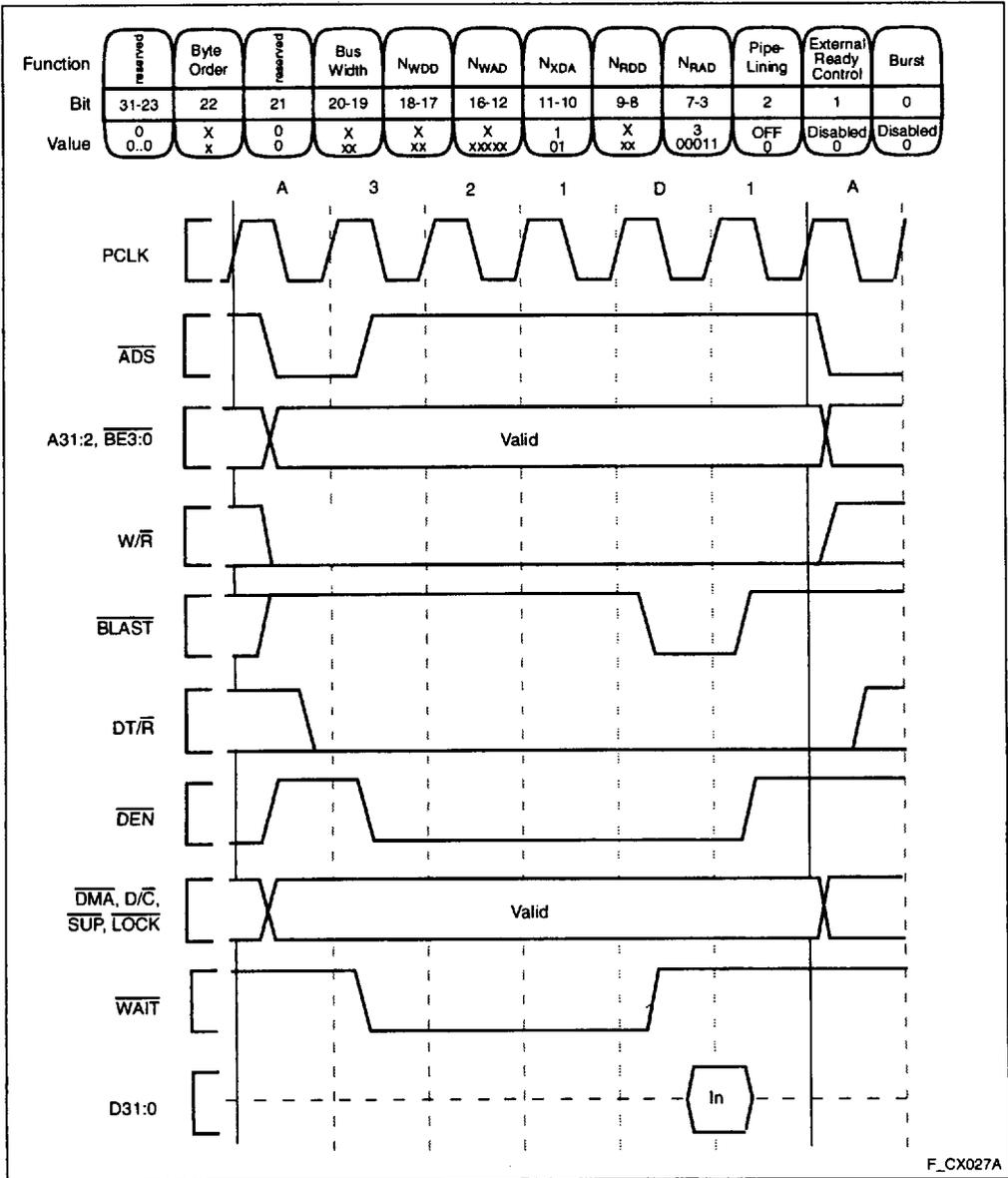
Figure 25. Non-Burst, Non-Pipelined Read Request With Wait States
