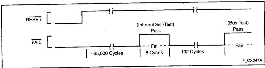
Figure 46. FAIL Functional Timing
