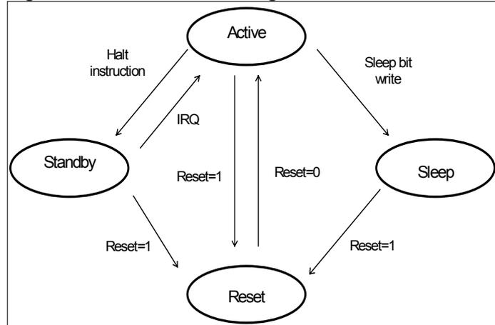
Sleep mode may be canceled only by a high level of min 10µs at the Reset terminal or by the selected port A input reset combination, if option **InpResSleep** in register **OPTFSeIPB** is turned on.
