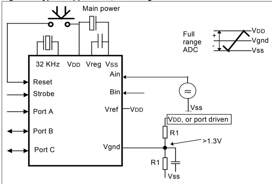
**Limited range ADC :**  $V_{DD} > V_{ref} > V_{gnd}$ ,  $V_{gnd} = V_{DD}/2$ .
