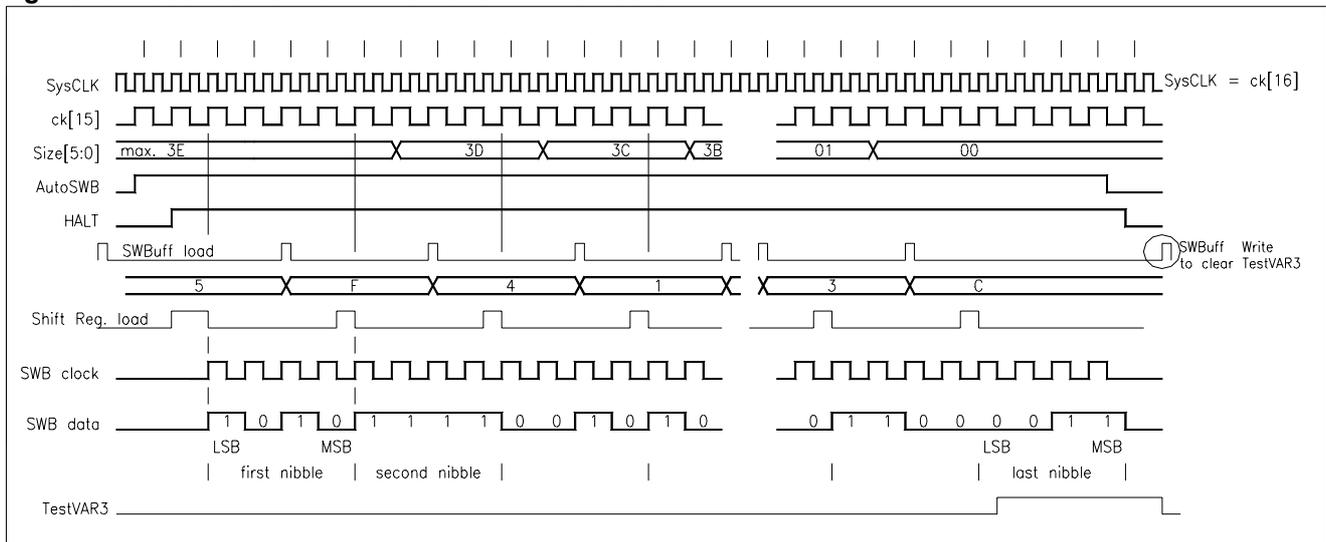
Because the data in the RAM are still present one can start transmitting the same data once again only by recharging the RegSWBuff, RegSWBSizeL and RegSWBSizeH register together with SWBAuto bit and putting the EM6517 in HALT mode. This will start a new transmission.
