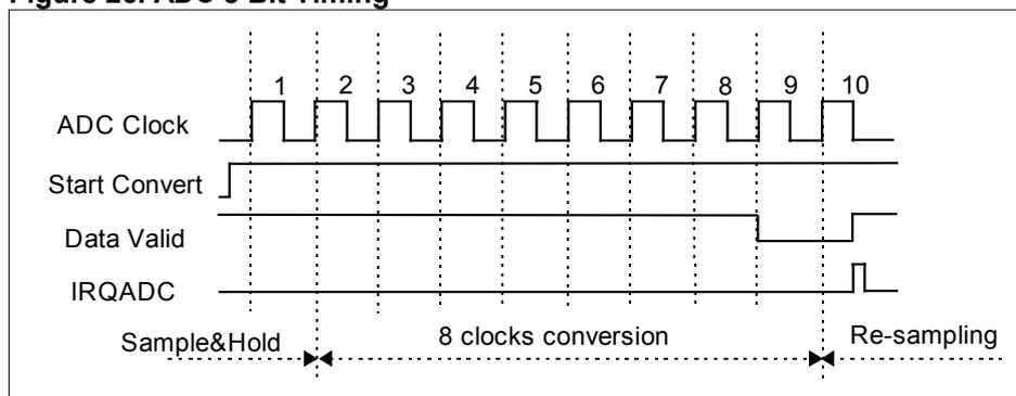
The ADC 8 bit contains an inherent sample and hold function : the input voltage is sampled during acquisition phase (2 clock cycles) and is held until the end of conversion. Total conversion time is 10 clock cycles.
