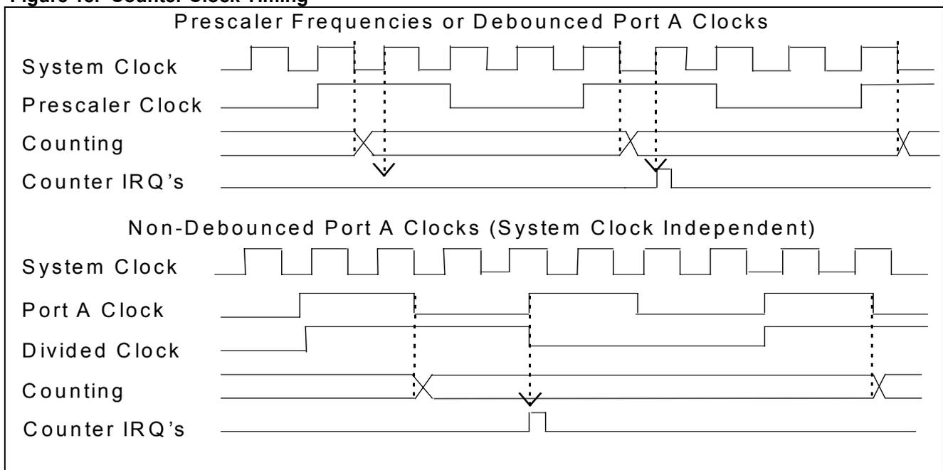
The two remaining clock sources are coming from the PA[0] or PA[3] terminals. Refer to the Figure 12 on page 14 for details. Both sources can be either debounced (Ck[11] or Ck[8]) or direct inputs, the input polarity can also be chosen. The output after the debouncer polarity selector is named PA3, PA0 respectively. For the debouncer and input polarity selection refer to chapter 7.2.4.
