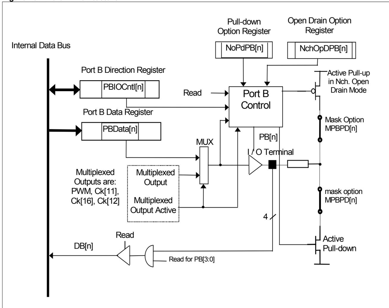
On each terminal of PB[3:0] an internal input pull-up (metal mask MPBPU[n]) or pull-down (metal mask MPBPD[n]) resistor can be connected per metal mask option. Per default the two resistors are in place. In this case one can chose per software to have either a pull-up, a pull-down or no resistor. See below.
