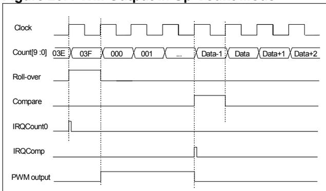
**Figure 21. PWM Output in Down Count Mode**
