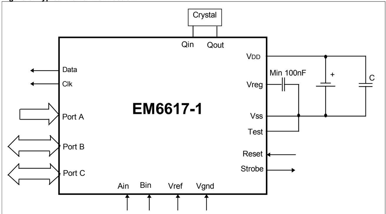
**Figure 7. Internal Power Connection**
