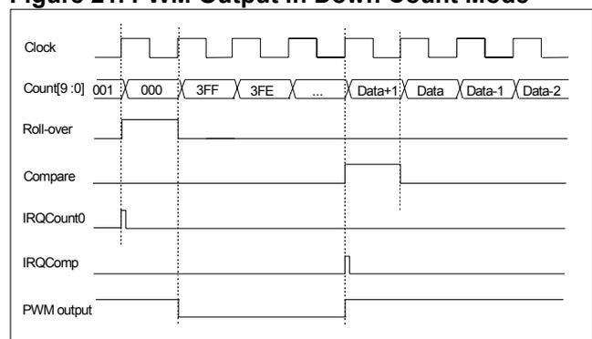
**In Down Count Mode** everything is inverted. The PWM output starts with the '1' value. Each Roll Over will set the output to '0' and each Compare Match will set it back to '1'. For limited pulse generation one must load the complementary pulse number value. I.e. for 5 pulses counting on 4 bits load bits[9 :4] with hex 3A (bin 111010).
