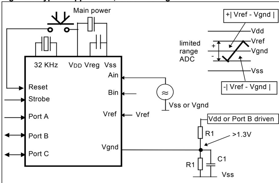
**other possibility:**  $V_{REF} = V_{regLogic}$ ,  $V_{GND} = V_{regLogic}/2$
