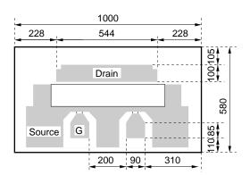
**Remark** Chip thickness:  $140 \mu m$  G : Gate
