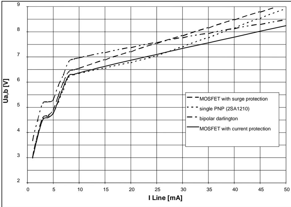
Fig. 9 shows a typical DC mask graph for the optional hook transistor arrangements: MOSFET with overcurrent protection, MOSFET with surge protection, single PNP and PNP darlington . The X-scale shows line current in mA and the Y-scale shows the voltage across the a- and b-terminals. Check with your application's PTT requirements to find the arrangement that fits best into the specification.
