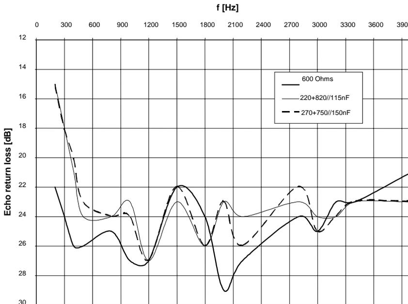
Fig.4 shows some typical results, measured with the DB1500I demo board with  $Z_{ref} = 600\Omega$ ,  $Z_{ref} = 220\Omega + 820\Omega//115nF$  and  $Z_{ref} = 270\Omega + 750\Omega//150nF$ . The board was configured as shown in the schematic, using a single bipolar (2SA1210) line transistor.
