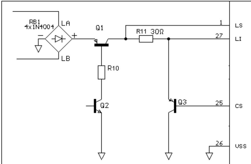
When going off-hook, SW1/1 short circuits the leakage supply resistor R1 and enables a low-ohmic path from line into the telephone. At the same time SW1/2 supplies the base of Q2 via R7 and R8 and signals a "off-hook" state to the IC's HS/DP-pin (#10). The base/gate of Q1 is pulled down by Q2 and the SA2532K is started up.  $V_{LI}$  (pin #27) is regulated to the specified voltage by shunt regulation from Q3. Line current flows through the following path:
