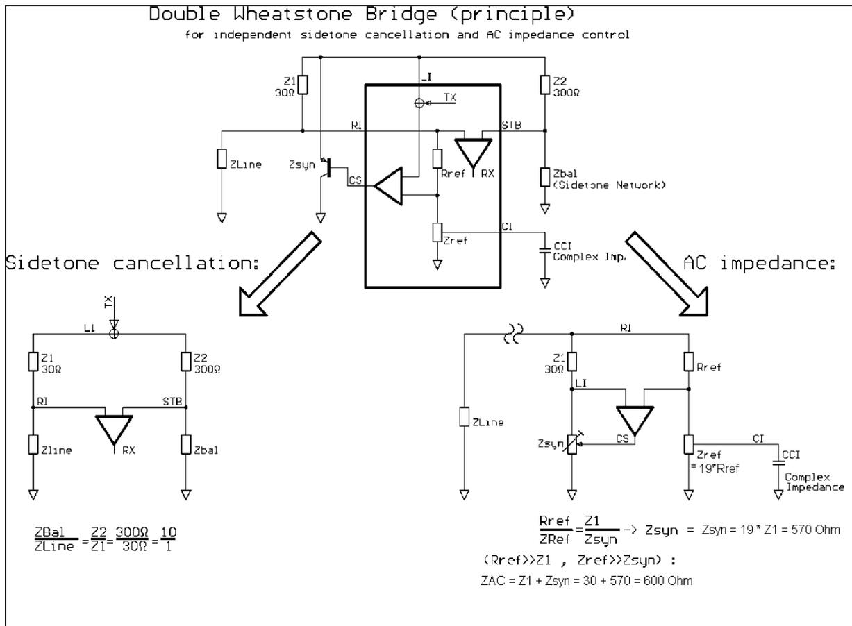
Fig. 5: Double Wheatstone bridge principle
