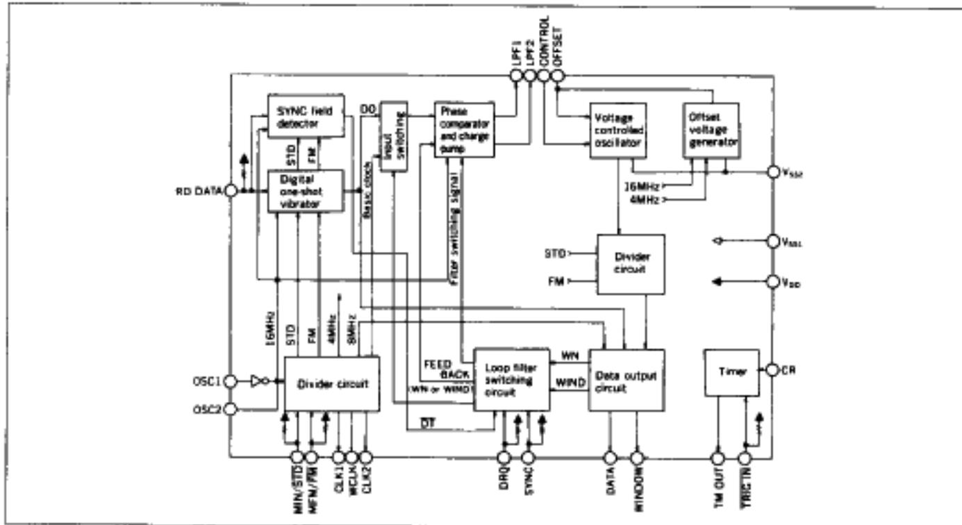
**■ PIN CONFIGURATION AND AN EXAMPLE OF EXTERNAL CIRCUITS**
