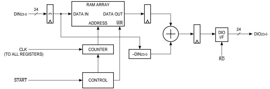
NOTE: NUMBER IN REGISTER INDICATES NUMBER OF PIPELINE DELAYS.
