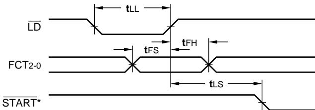
\*there must be at least one rising edge of CLK between the rising edge of LD and the falling edge of START\*.
