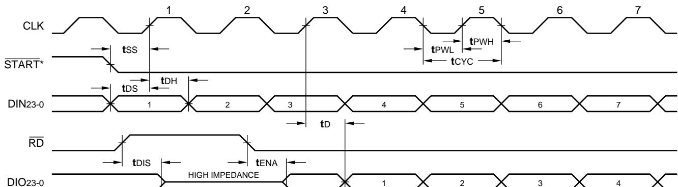
\*START must be held LOW a minimum of tSH after the rising edge of CLK that loads the last value of DIN23-0.
