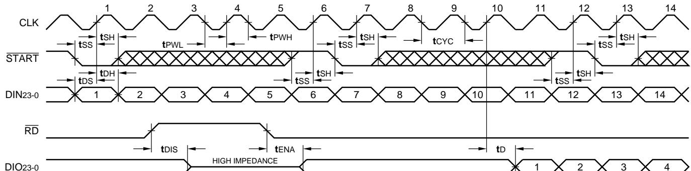
Shown are the waveforms for a delay length of 10.
