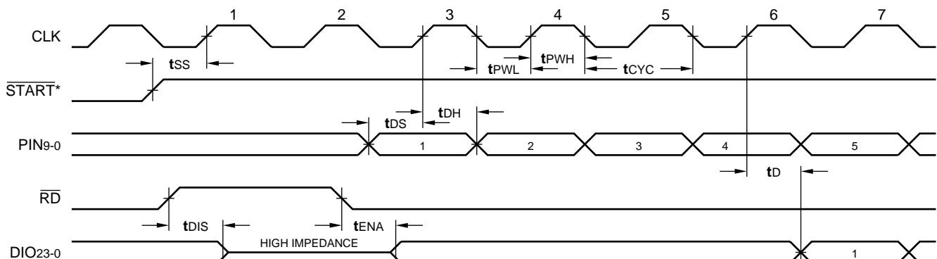
\*START must be held HIGH a minimum of tSH after the rising edge of CLK that loads the last value of PIN9-0.
